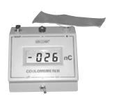
In a laboratory demonstration of the photoelectric effect, a sheet of zinc was placed on top of a coulombmeter and the zinc was given a negative charge.
